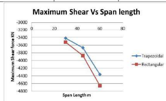
Figure 6: Maximum Shear force of different span length
