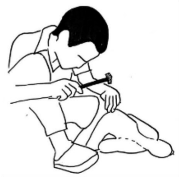
Figure 1. Repoussé Hammering on a Traditional Anvil
