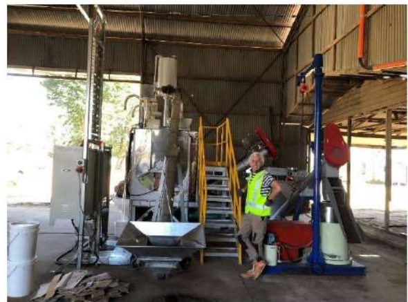
Figure 1: Rapid composting pilot plant set up for the monitoring of temperature and mixability in a thermophilic digester
