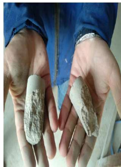
Figure 1: Brittle failure after testing of sample of high cement and epoxy resin content
