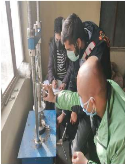
Figure 2: Unconfined Compressive Strength test of Samples
